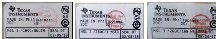
Figure 2. MSL 1,2,3 Rating and Peak Reflow Labeling Examples on Cardboard Box
