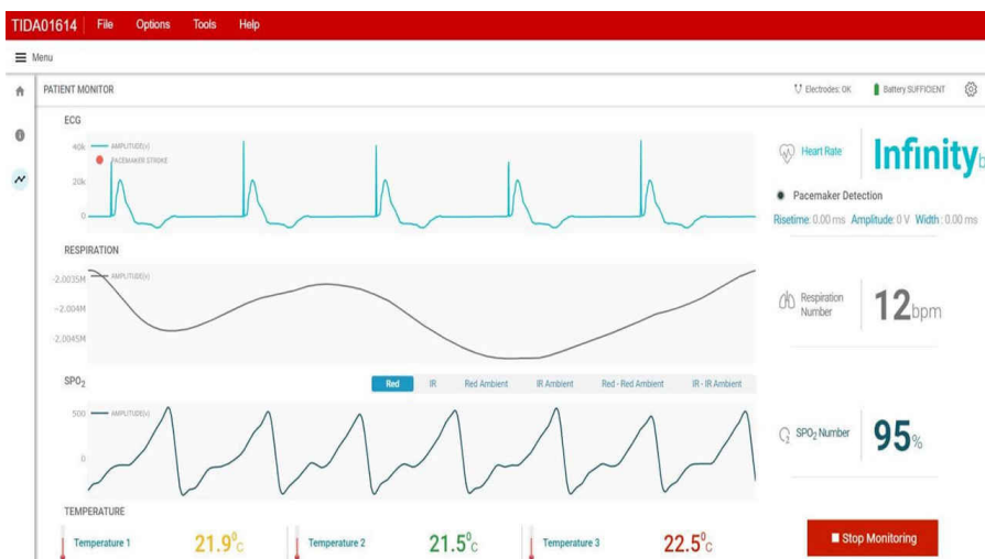
Figure 3. GUI Displaying ECG, PPG, Pacemaker, Heart Rate and Skin Temperature
