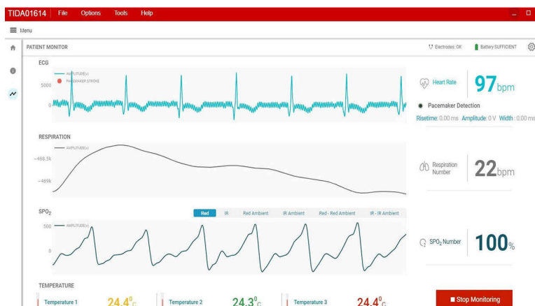
Figure 2. GUI Displaying ECG, PPG, Respiration, Heart Rate and Skin Temperature
